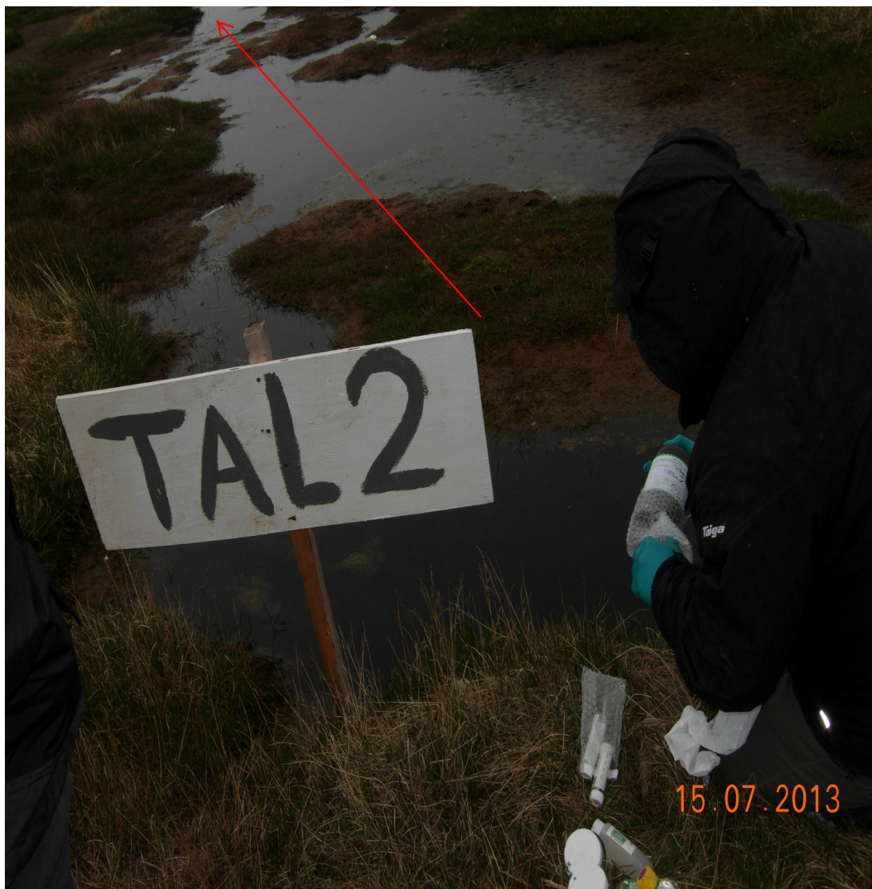
Picture4: Sewage effluent outfall from secondary cell (lagoon) onto wetland; 1 st sampling point.
