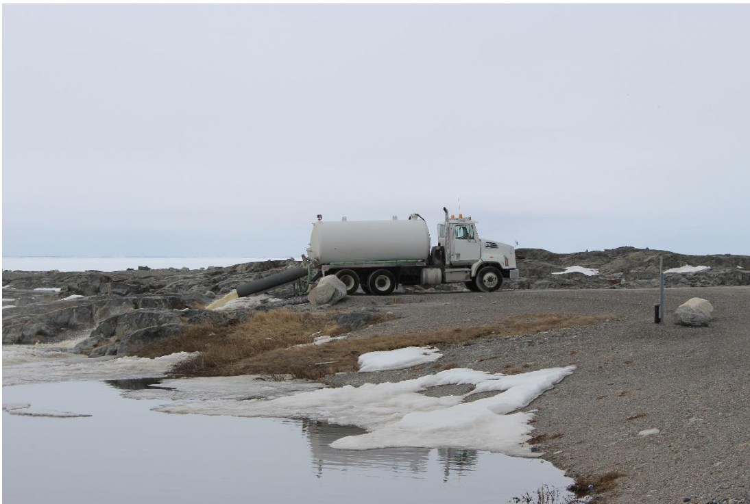
Figure 4 Discharging sewage truck
