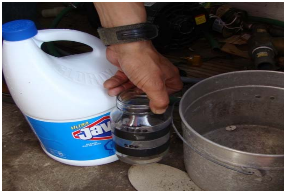
Photograph 7: Glass jar used to measure bleach for water treatment (photo taken Aug 1/08 during 2008 inspection)
