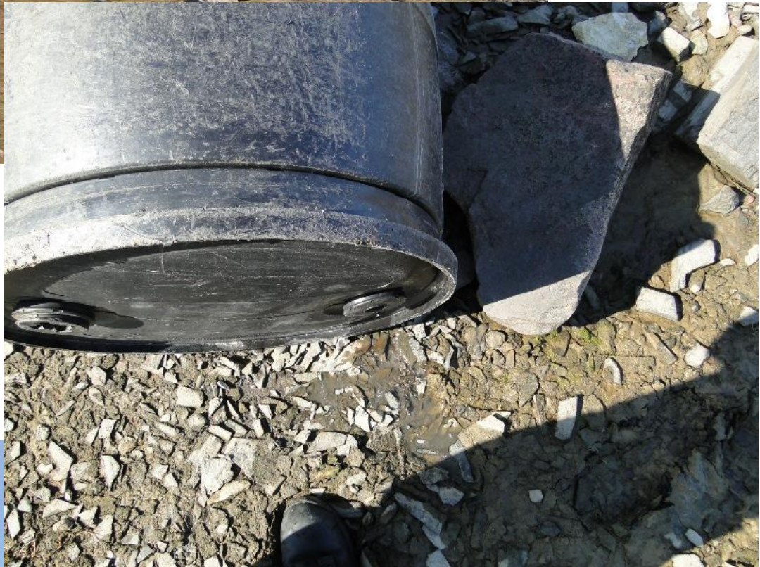
Figure 10. Water coming out of barrel smells of hydrocarbons.
