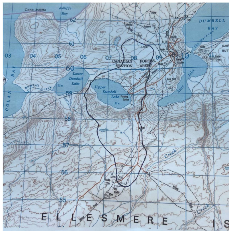
Figure 1: 1:50,000 topographic map of the Alert, NU region, including Upper Dumbell Lake. Dark outline is sketching of approximate watershed boundary based on topographic contours.
