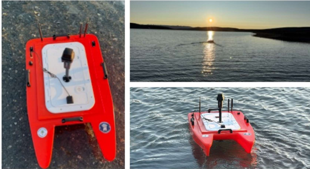
Figure 5: One-day testing of the BathyLogger system on Upper Dumbell Lake. Clockwise from left: Bathylogger system at shore (notice thin ice and surface bubble in above boat); Bathylogger system motoring toward a low-horizon Sun; Bathylogger system returning to shore. Upper Dumbell Lake froze over the following day, preventing us from completing the bathymetric survey in 2025.
