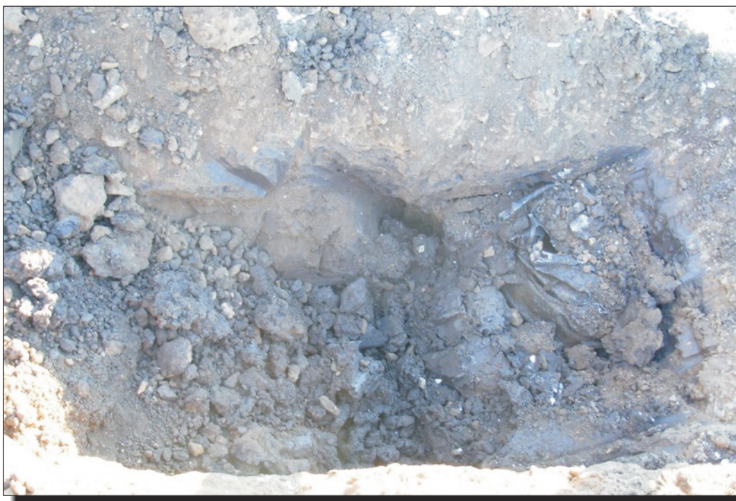
Photo 8 Area 3, DND Barrel Landfill - test pit encounter with crushed fuel drum.
