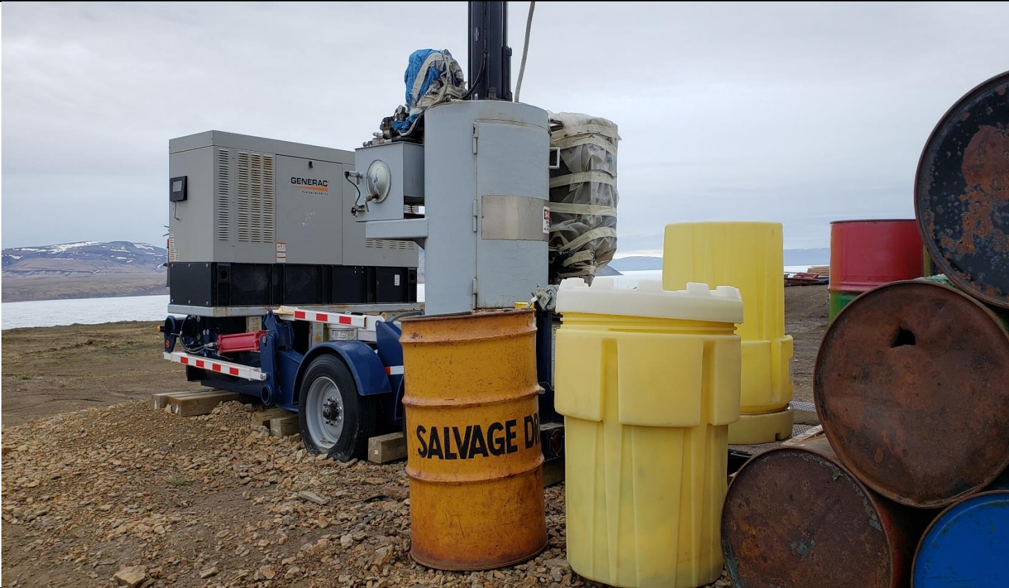
Description: Drum washer and crusher. After washing a drum, it is suitable for burial underground.
