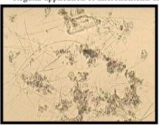
micronutrients will shorten the "lag phase" and speed the recovery of a system that has experienced a toxic shock or increased loading.
