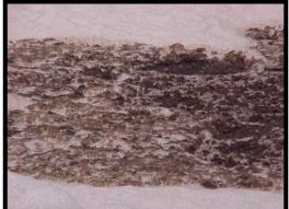
In a papermill, sometimes the foam looks a bit brown. Check to make sure it does not mean the bacteria are older, but it may mean that your primary is not capturing all the fiber. Did you know a 1% fiber capture recovery could mean up to a million dollars a year if returned back to the front end? Make sure your primary is doing the job correctly. See troubleshooting chart on foam and colors. Better capture in the primary also helps with TSS and BOD loading on the pond.
