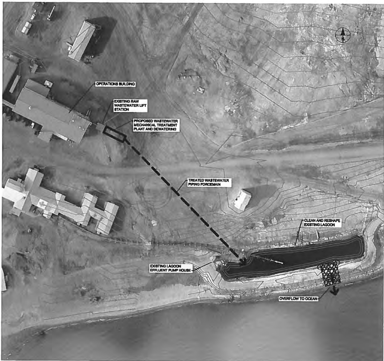
Figure 3: Wastewater Discharge Pipe and Detention Basin
