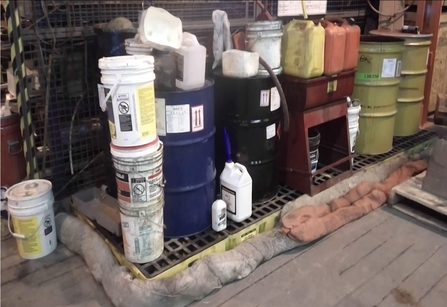
Description: Hazardous Materials, and waste storage and transfer station. Material is stored in secondary containment, and with hydrocarbon booms to capture any small spills.
