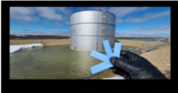
Photo E 1: Hydrocarbon test strips used in berm of tank W22A (19-Jun-2020)
