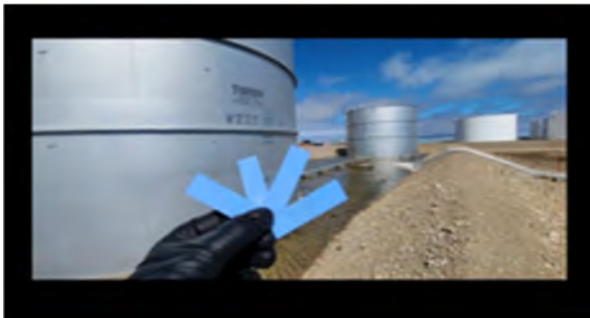
Photo E 3: Hydrocarbon test strips used in berm of tank W22C & W20D (19-Jun-2020)
