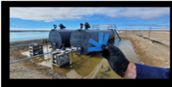
Photo E 2: Hydrocarbon test strips used in berm of tank W20B & W20C (19-Jun-2020)
