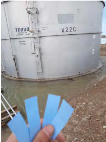
Photo E 3: Hydrocarbon test strips used in berm of tank W22C & W20D (18-Jun-2021)
