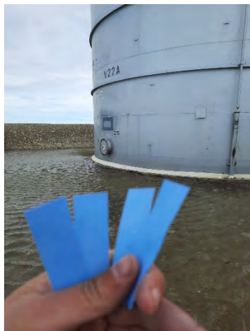
Photo E 1: Hydrocarbon test strips used in berm of tank W22A (18-Jun-2021)
