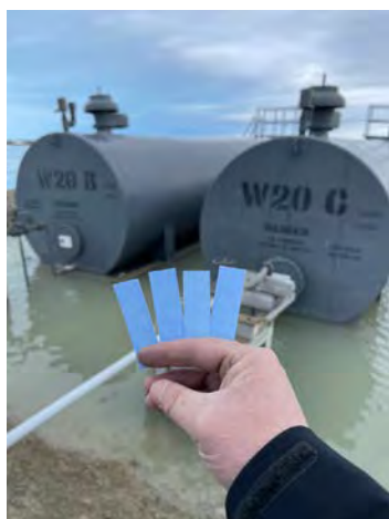
Photo E 2: Hydrocarbon test strips used in berm of tank W20B & W20C (18-Jun-2021)
