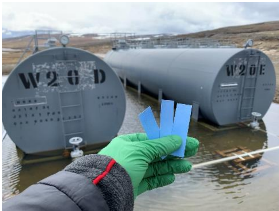
Photo E 4: Hydrocarbon test strips used in berm of tank W20D &amp; W20E (8-Jul-2021)
