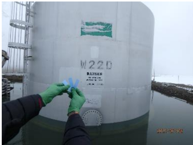
Photo E 3: Hydrocarbon test strips used in berm of tank W22D (8-Jul-21)
