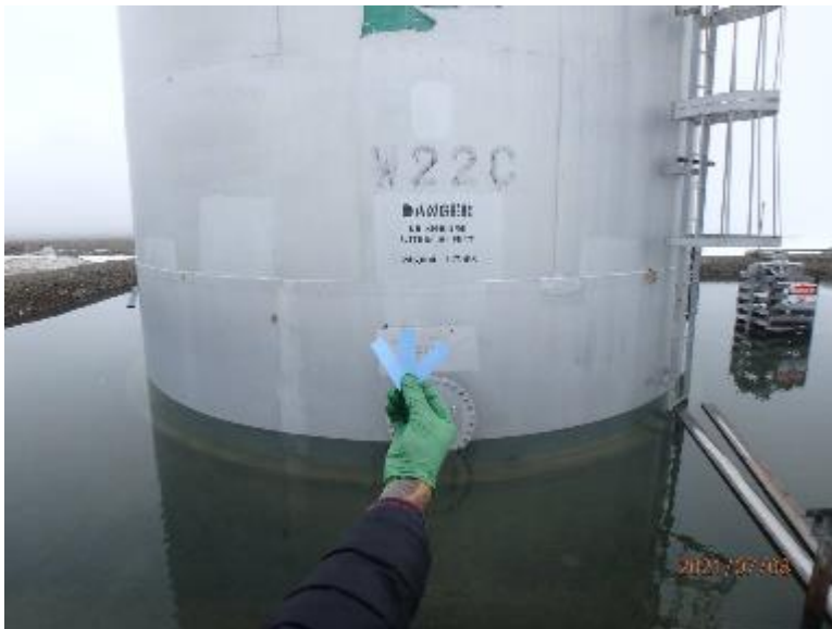
Photo E 2: Hydrocarbon test strips used in berm of tank W22C (8-Jul-21)
