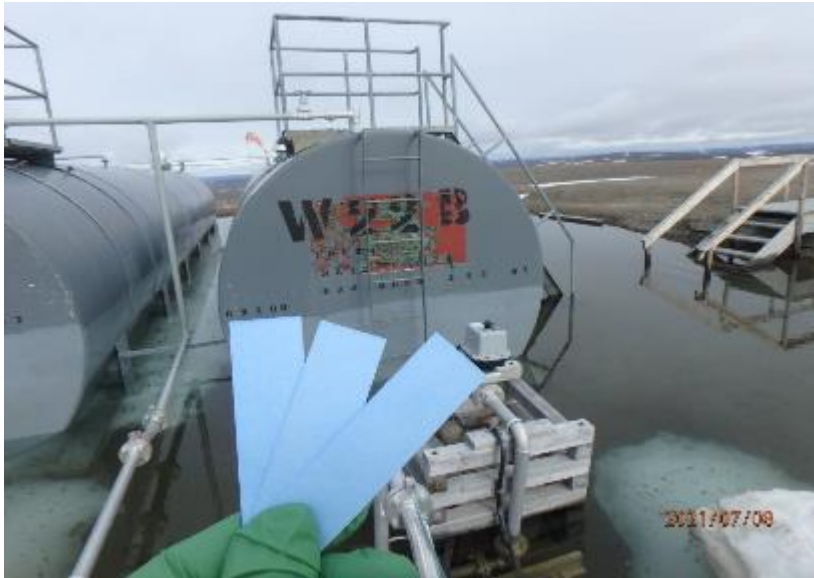
Photo E 1: Hydrocarbon test strips used in berm of tanks W22A & W22B (8-Jul-21)
