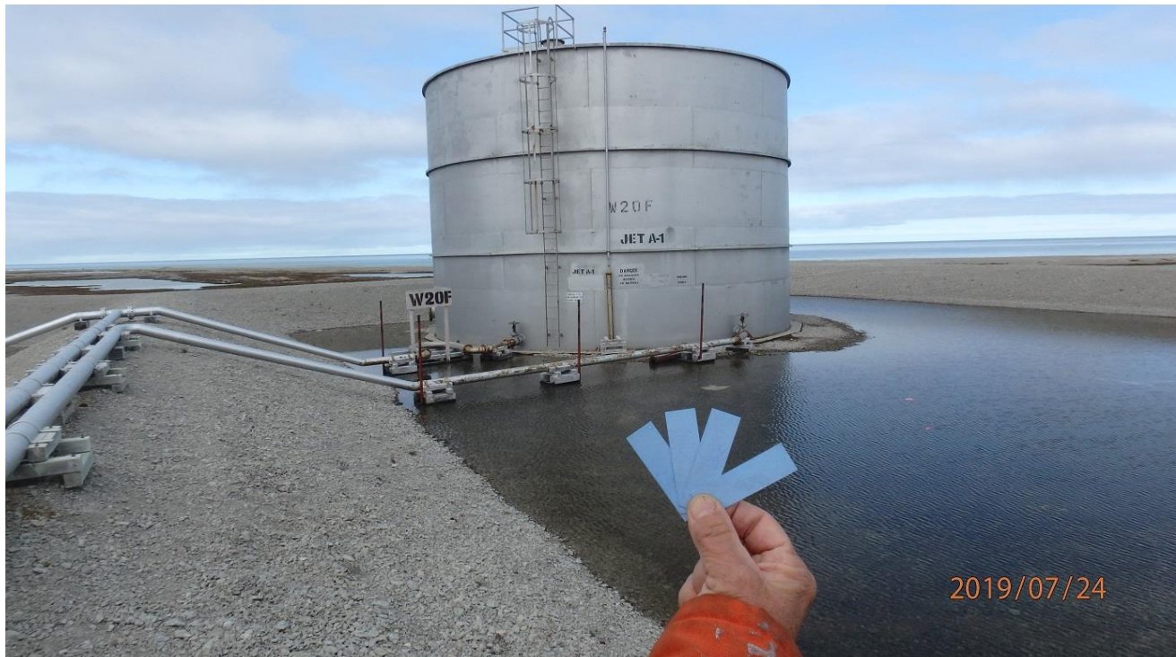
Figure 44: Hydrocarbon test strips used in the berm of tank W22F (24-Jul-2019)
