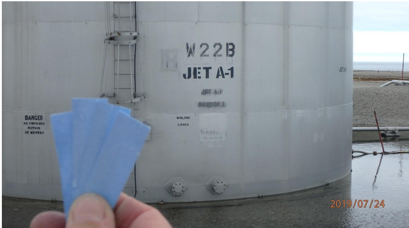
Figure 43: Hydrocarbon test strips used in the berm of tank W22B (24-Jul-2019)
