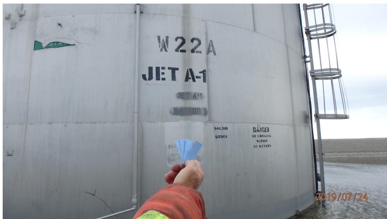
Figure 42: Hydrocarbon test strips used in berm of tank W22A (24-Jul-2019)
