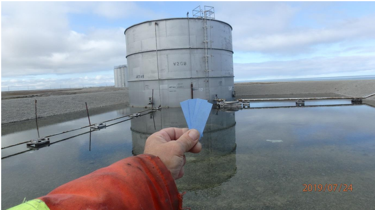
Figure 45: Hydrocarbon test strips used in the berm of tank W20B (24-Jul-2019)
