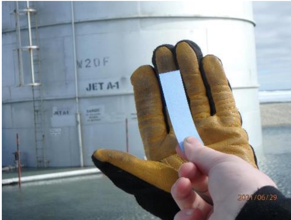
Photo E 7: Hydrocarbon test strips used in berm of tank W20F (29-Jun-2021)
