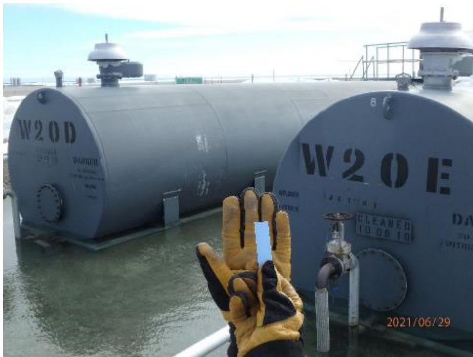
Photo E 5: Hydrocarbon test strips used in berm of tank W220D &amp; W20E (29-Jun-2021)
