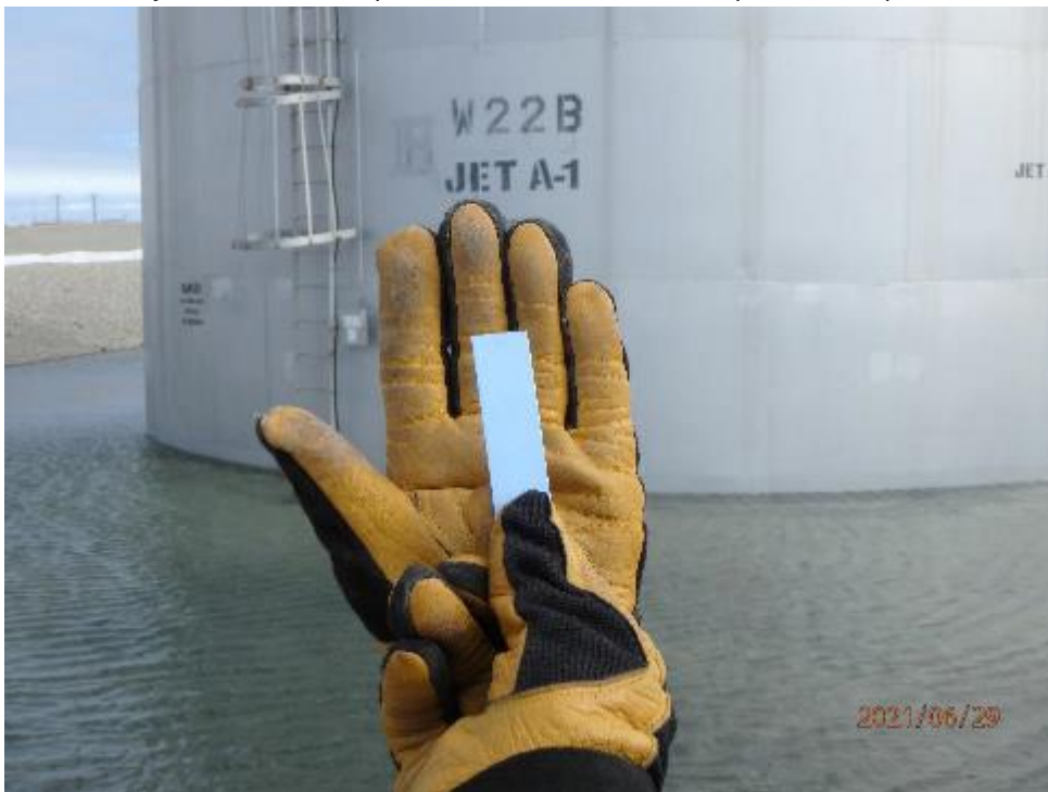
Photo E 10: Hydrocarbon test strips used in berm of tank W22B (29-Jun-2021)
