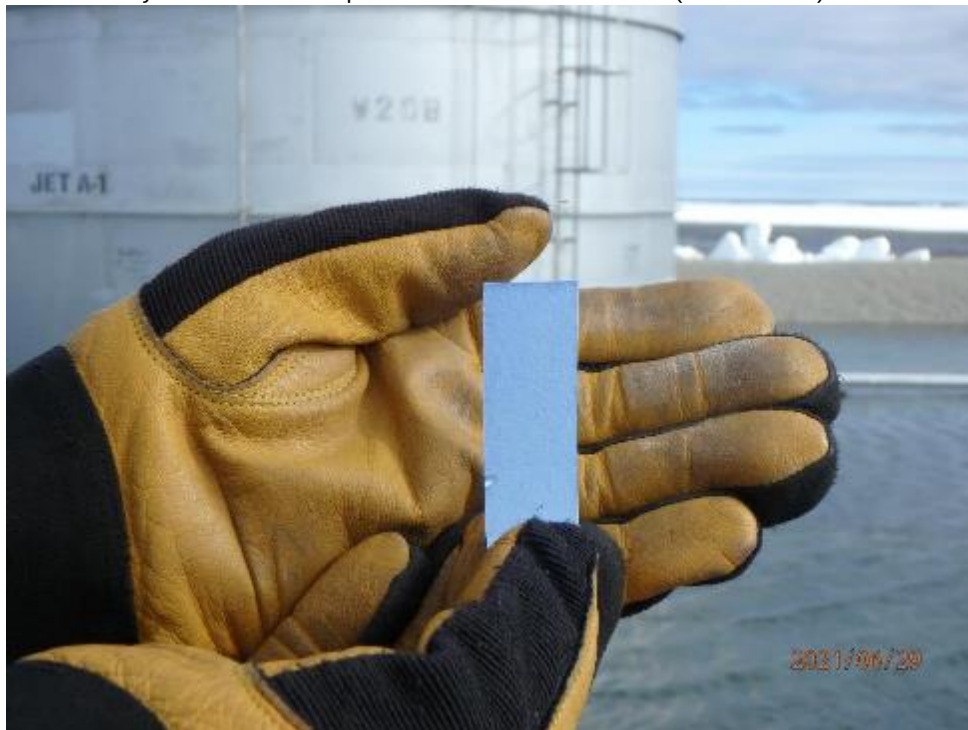
Photo E 3: Hydrocarbon test strips used in berm of tank W20B (29-Jun-2021)
