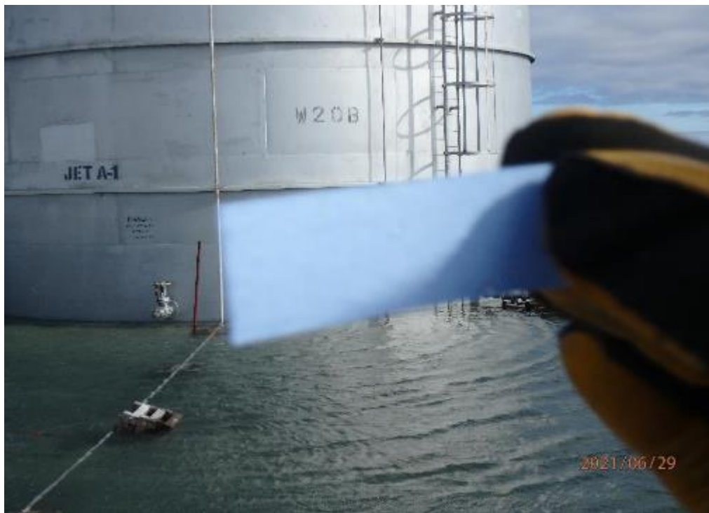
Photo E 2: Hydrocarbon test strips used in berm of tank W20B (29-Jun-2021)
