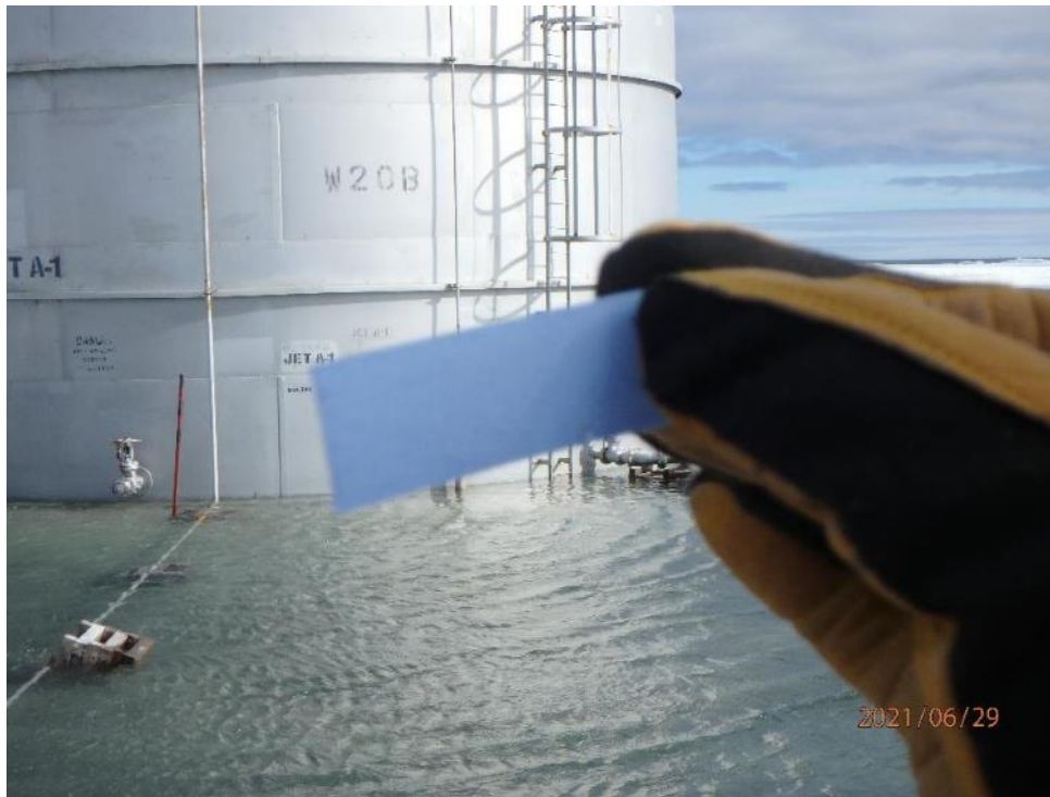
Photo E 1: Hydrocarbon test strips used in berm of tank W20B (29-Jun-2021)
