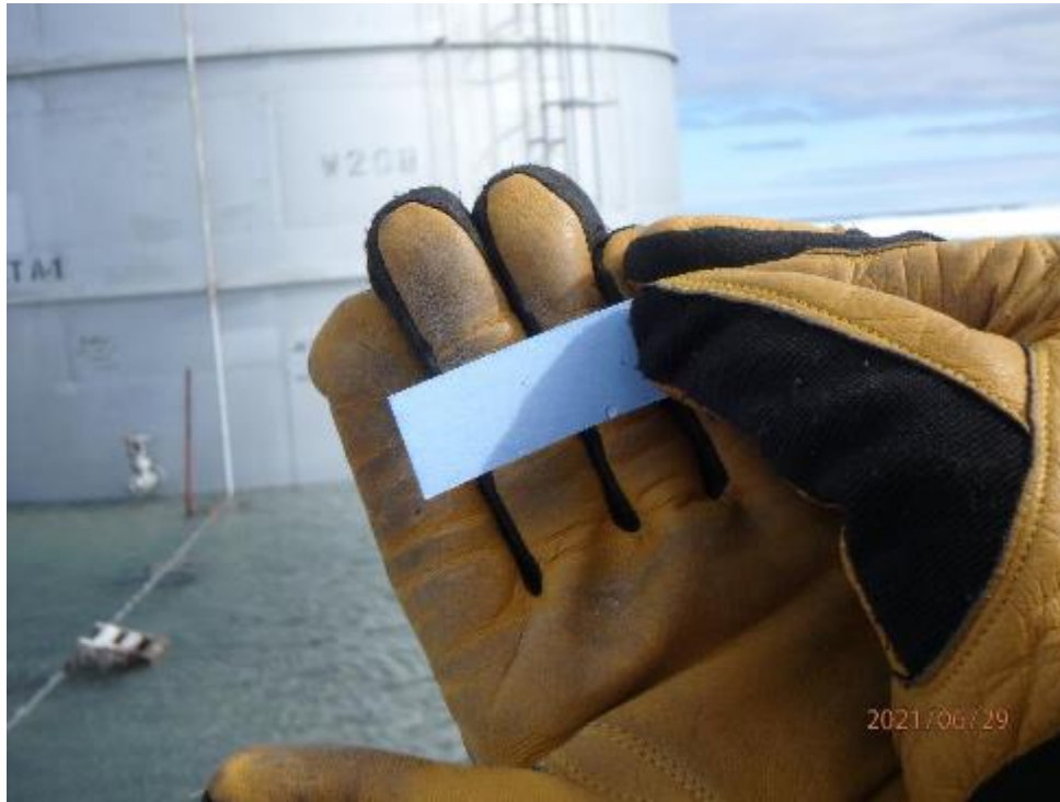
Photo E 3: Hydrocarbon test strips used in berm of tank W20B (29-Jun-2021)
