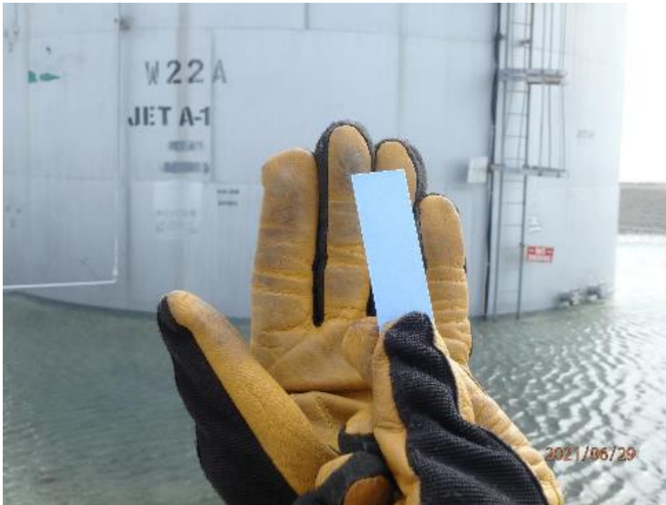
Photo E 9: Hydrocarbon test strips used in berm of tank W22A (29-Jun-2021)
