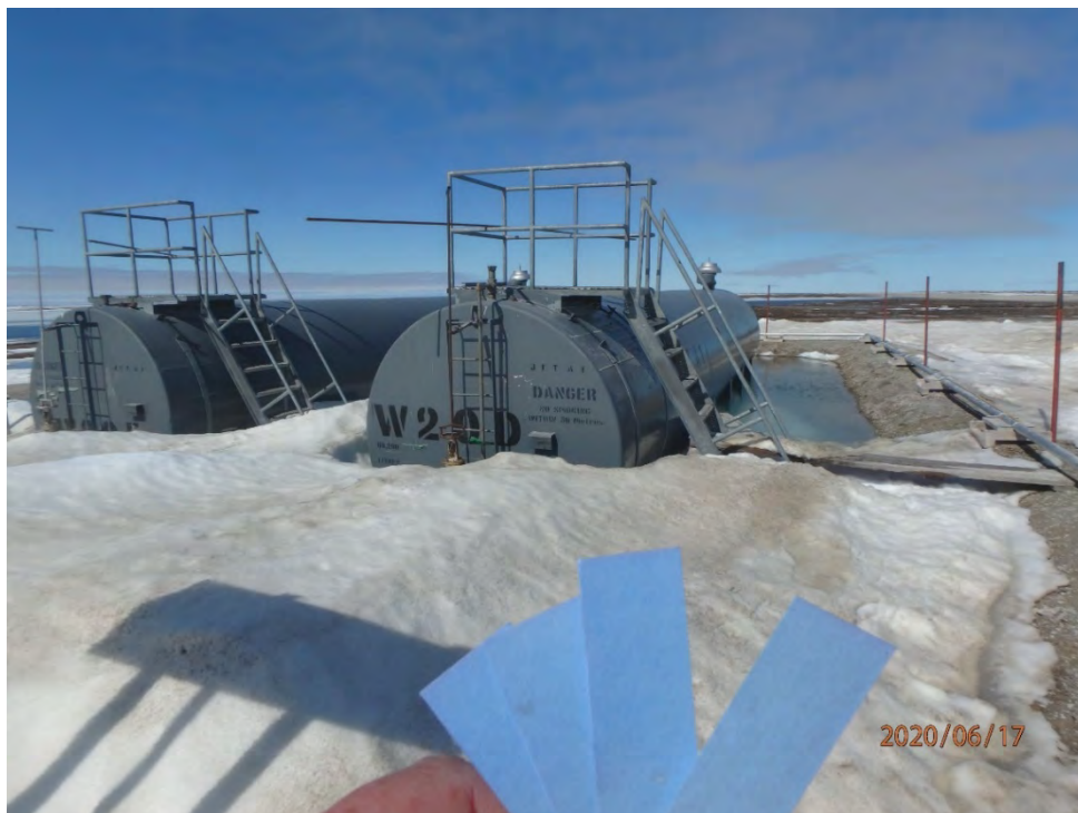
Photo E 3: Hydrocarbon test strips used in berm of tank W20D (17-Jun-2020)
