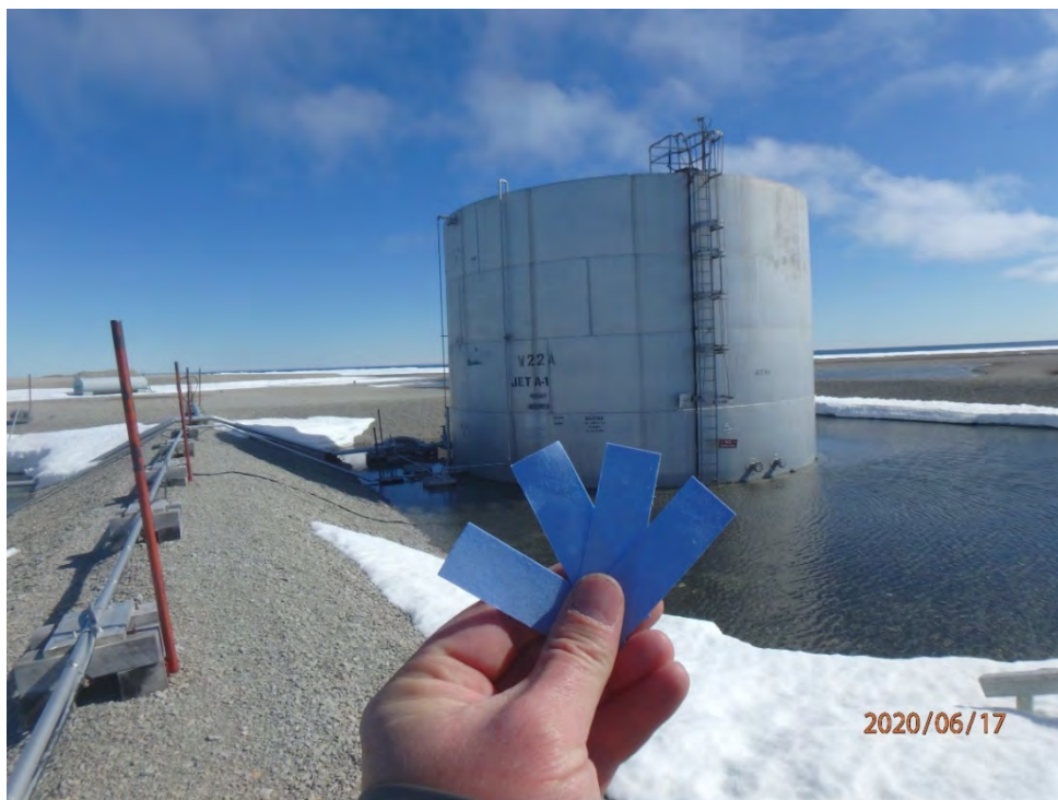
Photo E 4: Hydrocarbon test strips used in berm of tank W22A (17-Jun-2020)
