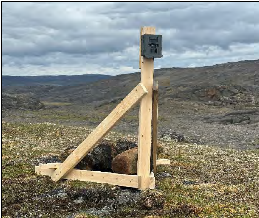
Plate 4.1-1. Example of a wildlife camera installed on a 2x4 stand in the project area
