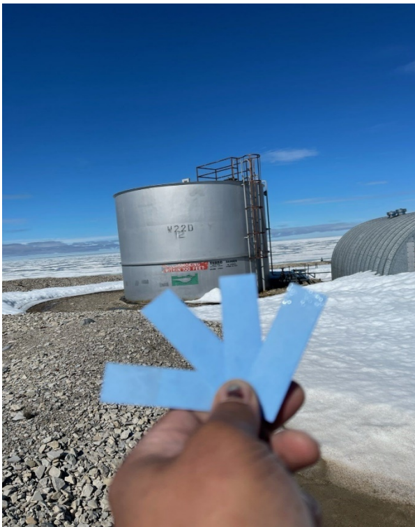
Photo E 2: Hydrocarbon test strips used in berm of tank W22D (12-Jul-2021)
