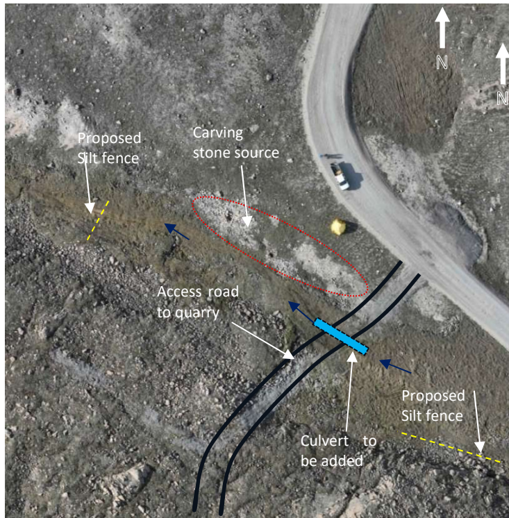
Figure 1.5.2: Culvert to be added
