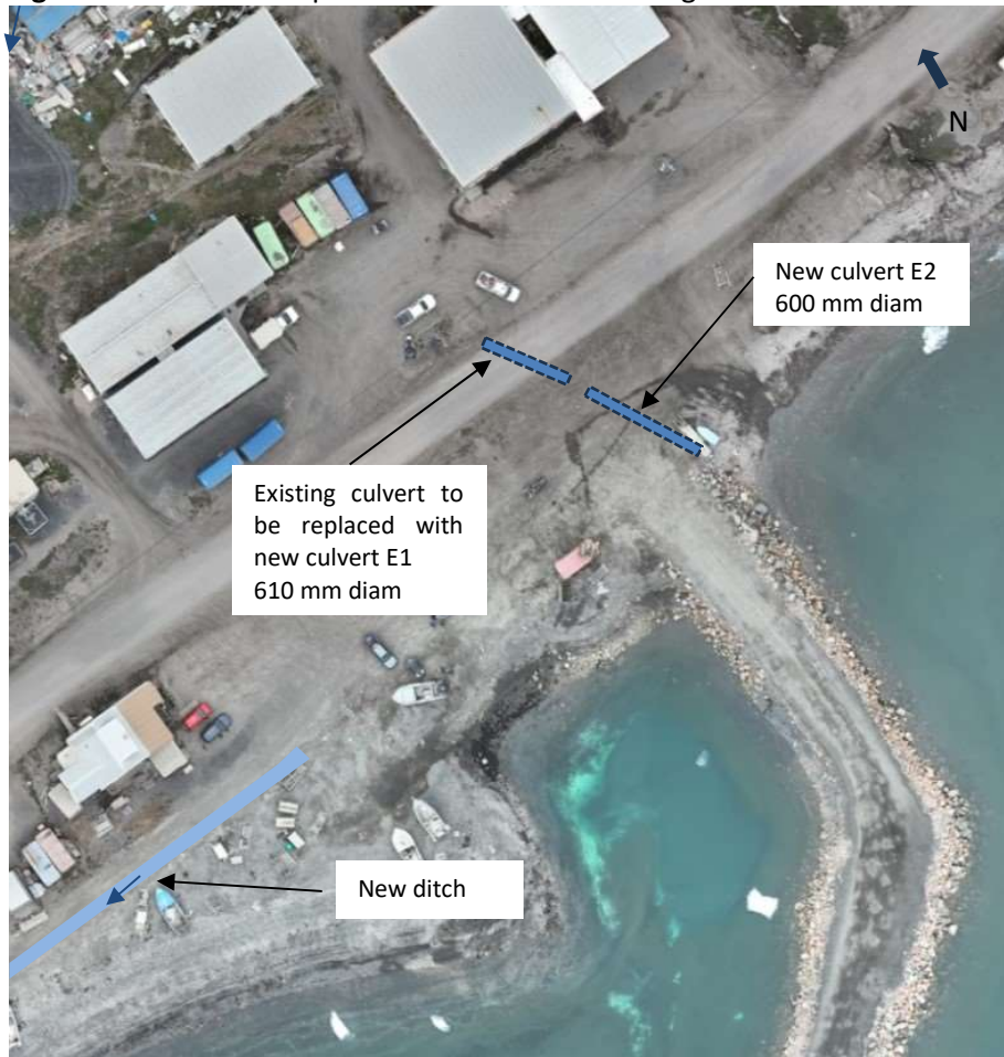
Figure 2.6.2: Culvert replacement under the existing road and new culvert to be added
