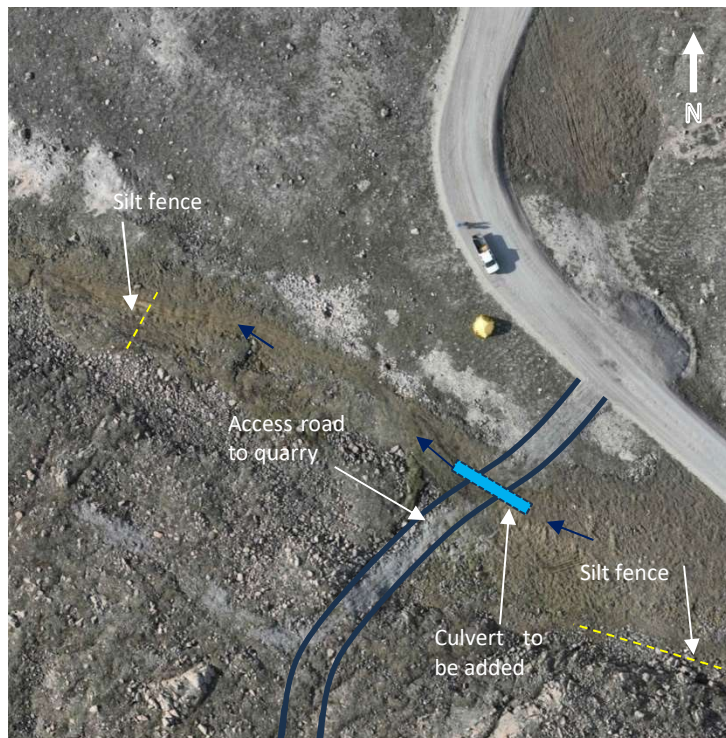
Figure 2.1.3 : Culvert to be added
