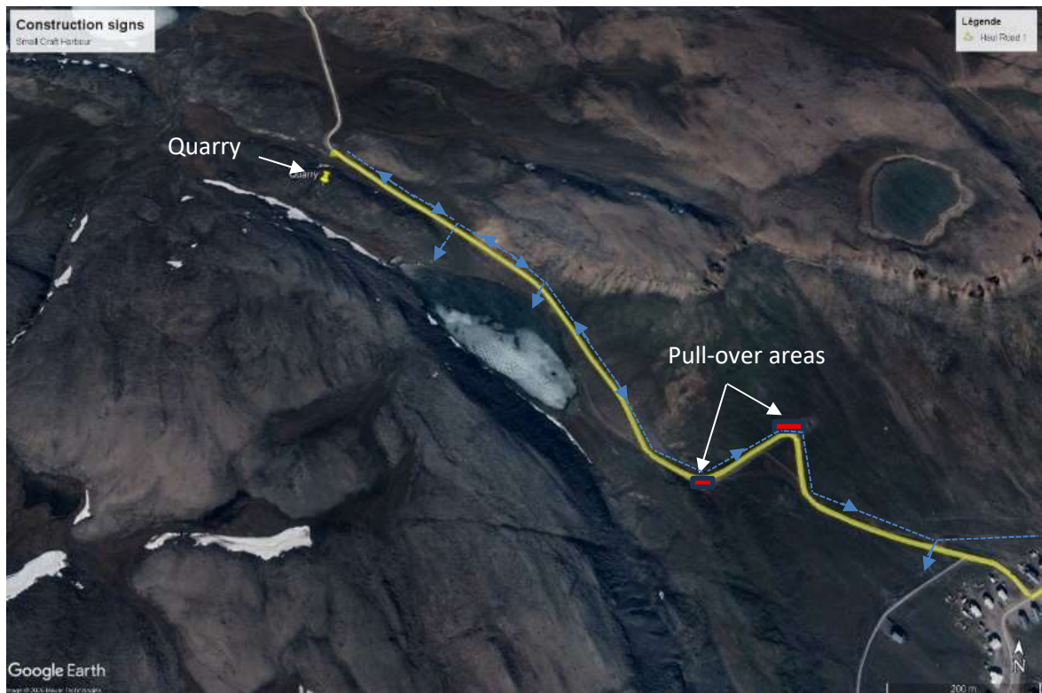
Figure 2.3.1: Haul road from the quarry to the construction site
