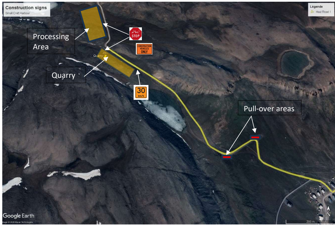
Figure 4.2.1 Hauling Road Construction Signs
