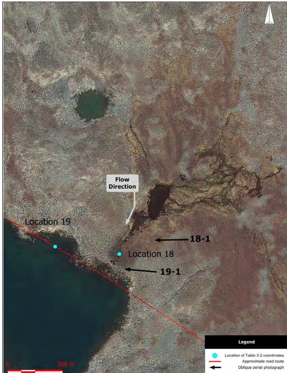
Locations 18 and 19. Aerial photograph (scale 1:5000) showing the approximate road route, the location of coordinates provided in Table 3-2, the flow direction, and the location of oblique aerial photographs. Lake at Location 19 will be avoided.
