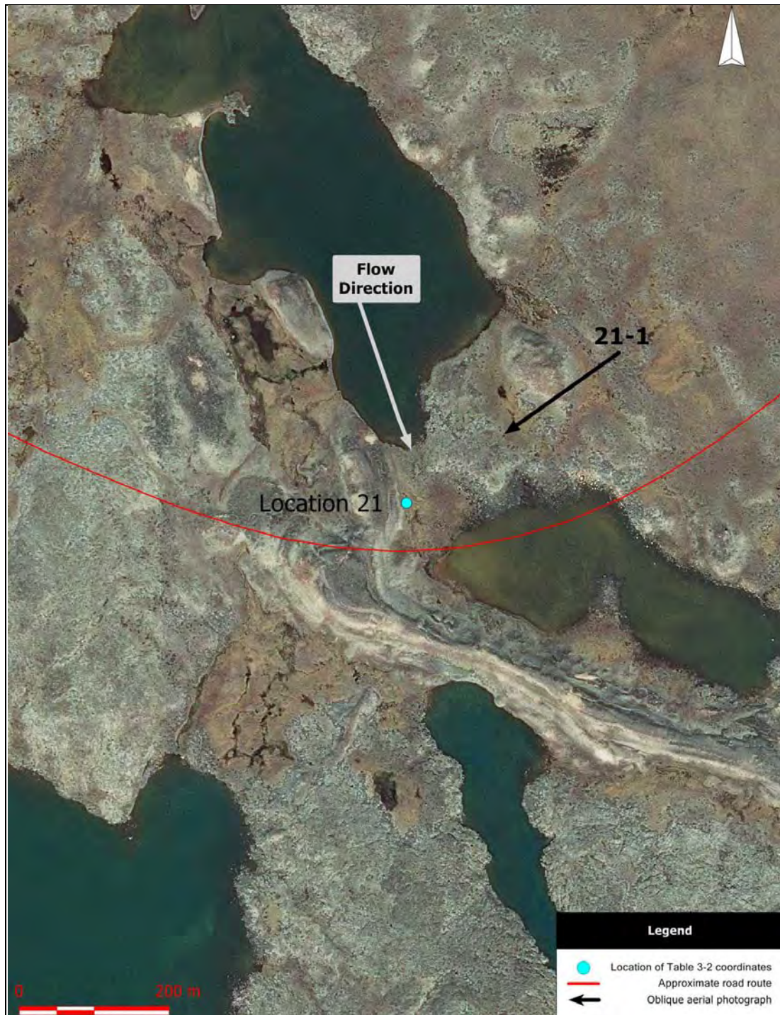
Location 21. Aerial photograph (scale 1:5000) showing the approximate road route, the location of coordinates provided in Table 3-2, the flow direction, and the location of oblique aerial photographs. Lake near Location 21 will be avoided.
