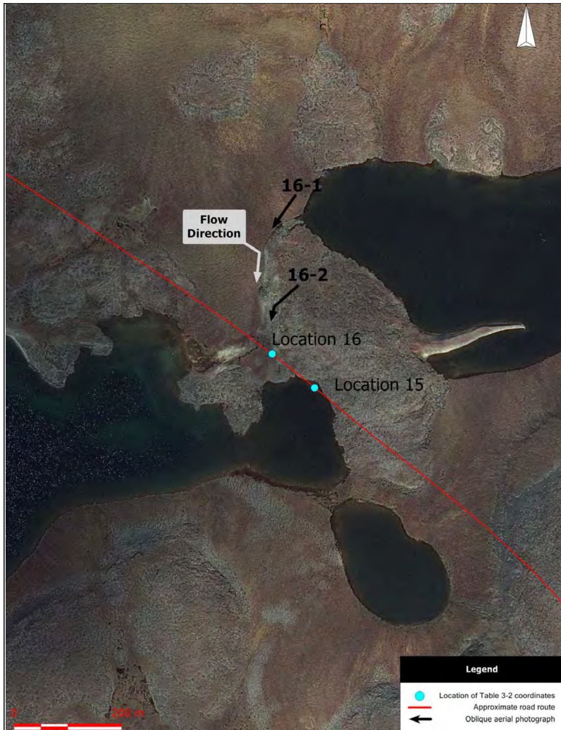
Locations 15 and 16. Aerial photograph (scale 1:5000) showing the approximate road route, the location of coordinates provided in Table 3-2, the flow direction, and the location of oblique aerial photographs. Lake at Location 15 will be avoided.
