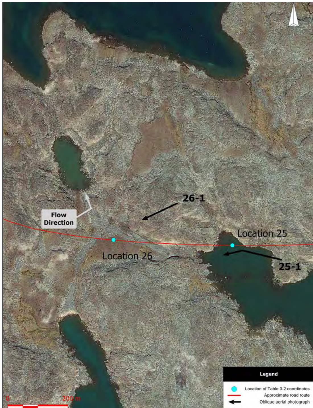
Locations 25 and 26. Aerial photograph (scale 1:5000) showing the approximate road route, the location of coordinates provided in Table 3-2, the flow direction, and the location of oblique aerial photographs. Lake at Location 25 will be avoided.
