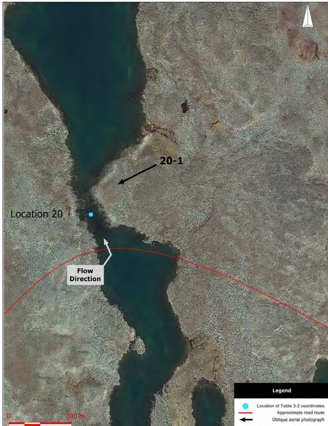
Location 20. Aerial photograph (scale 1:5000) showing the approximate road route, the location of coordinates provided in Table 3-2, the flow direction, and the location of oblique aerial photographs. Lakes near Location 20 will be avoided.
