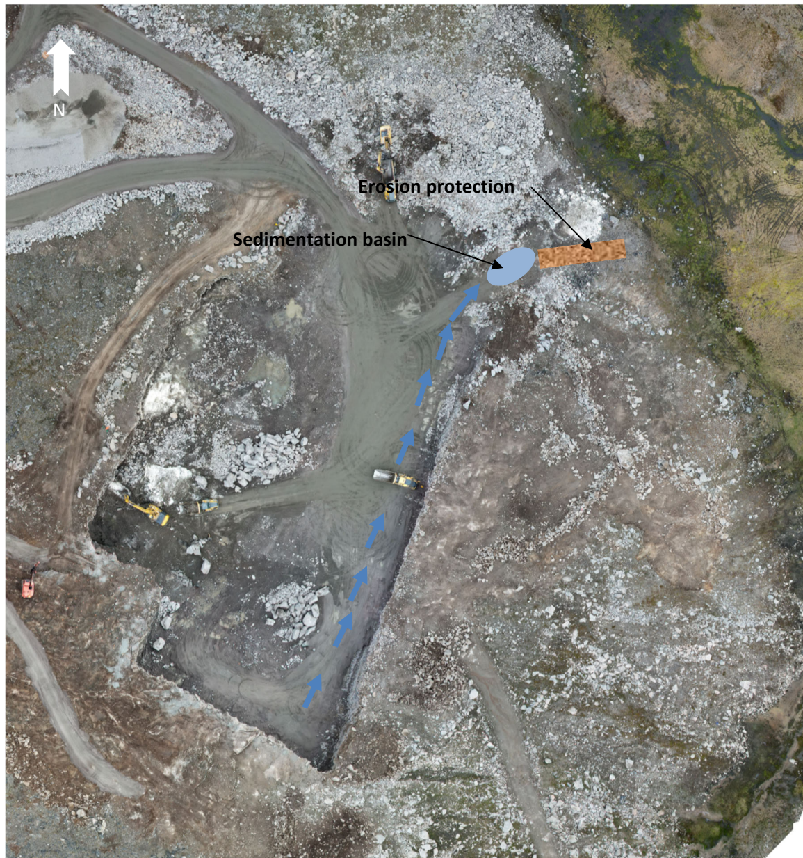
Figure 2.1.1: Erosion and sediment control measures to be constructed at the quarry
