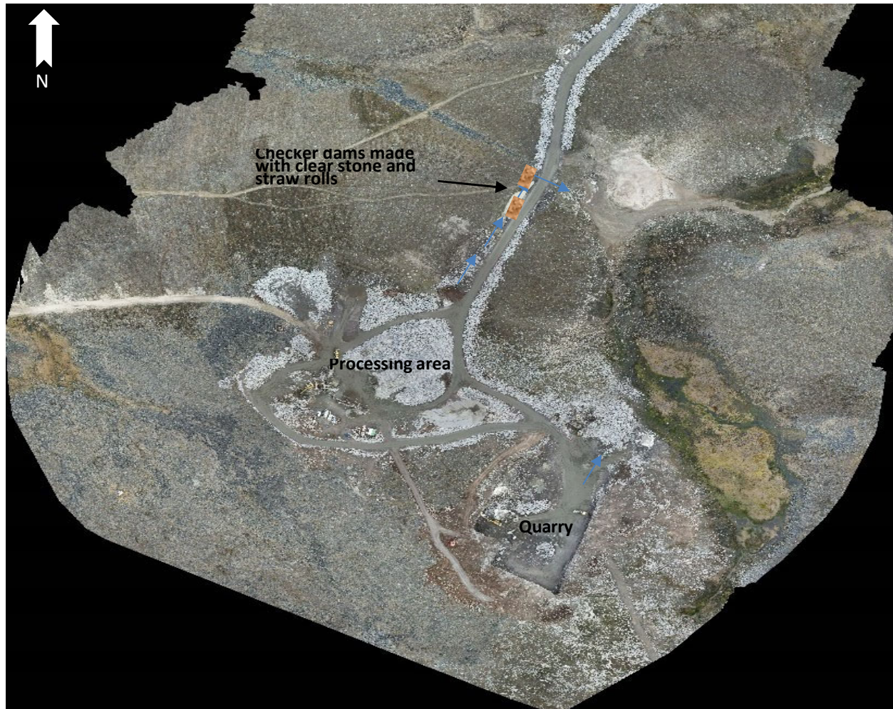
Figure 2.2.1: Erosion and sedimentation protection -Material processing area
