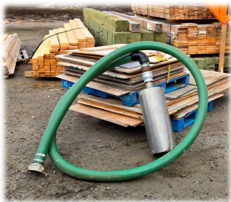
Fish Screen Installed at the End of the Intake Hose for Pumping Water into the River
