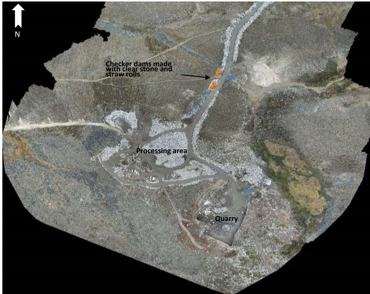
Figure 2.2.1: Erosion and sedimentation protection -Material processing area
