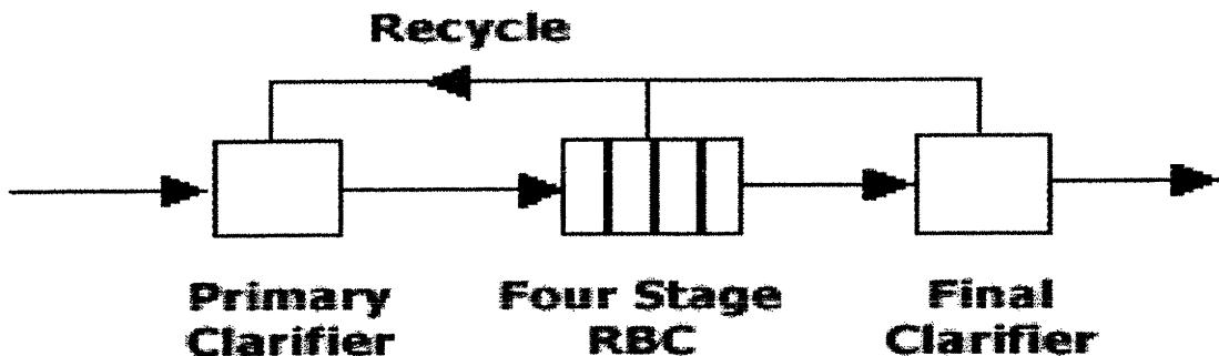
The Biodisk process requires a primary clarifier. The primary allows FOG to float, store sludge for 9 months, add heat and promote process stability.
