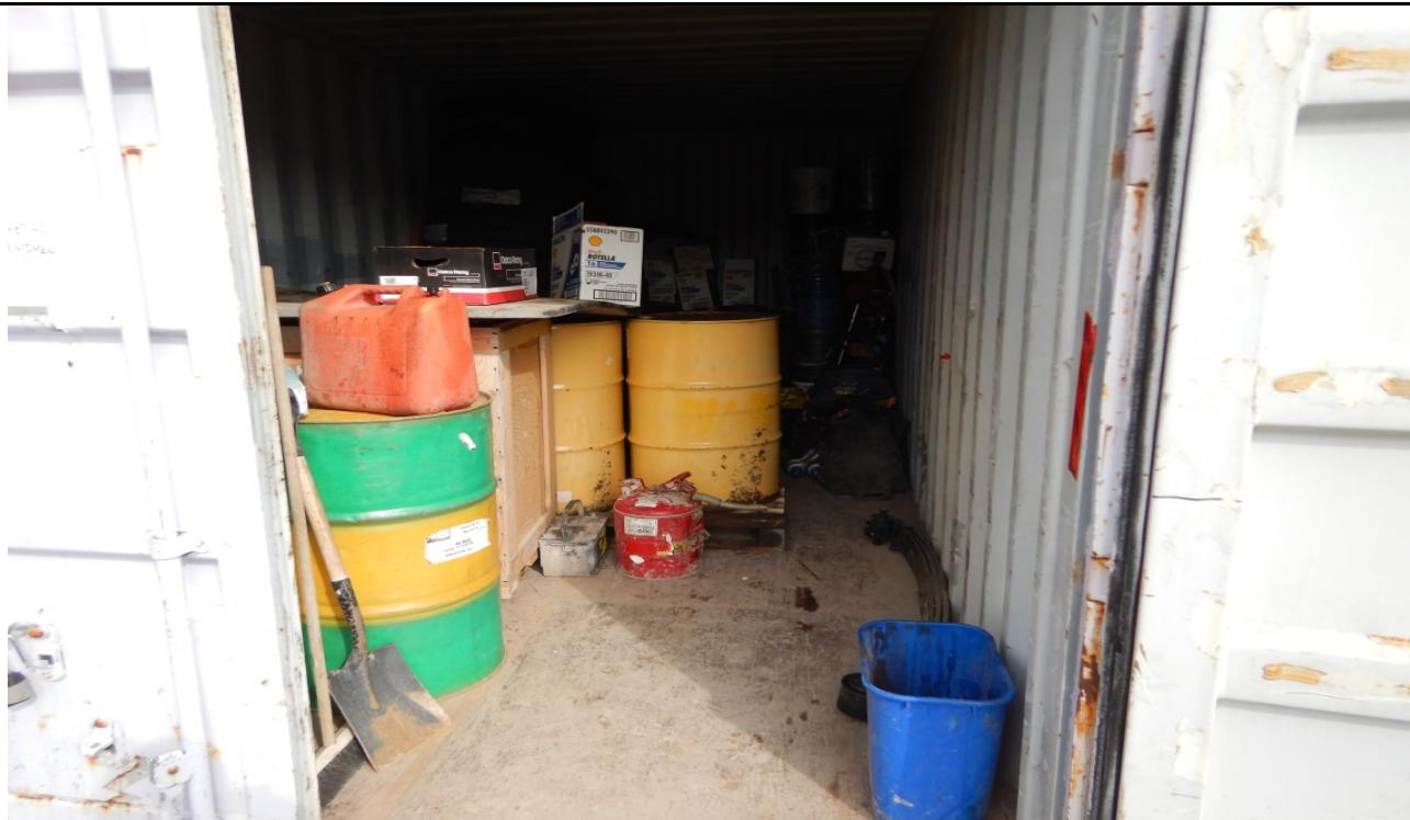
Description: hazardous Waste station – hazardous waste barrels in secondary containment in sea can encapsulated from the outside elements.
