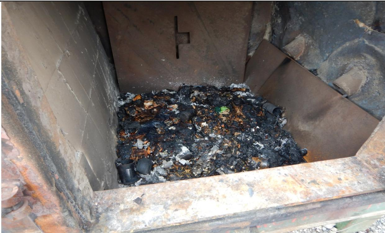
Description: Incinerator – Lots of signs of metal burnt in incinerator
