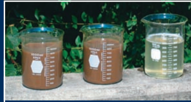
Sludge before (left) and after (right) treatment with Geotube® dewatering technology.
