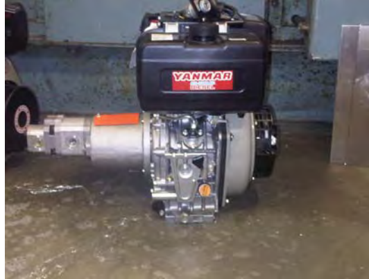
Figure 2: The gear pump and engine. The pump is mounted on the engine casing.
