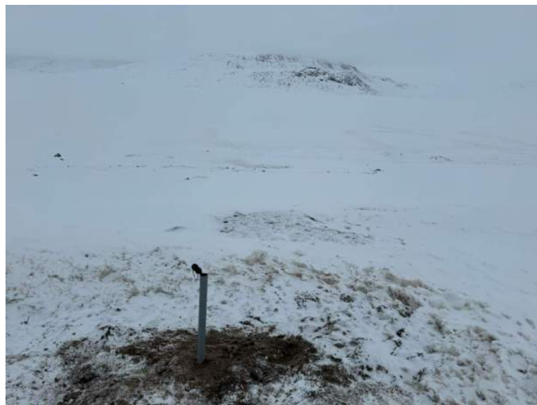
Photograph 10 Thermistor T4 installed in BH13.
