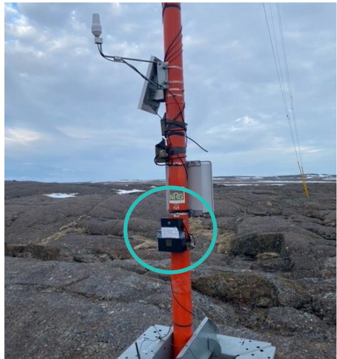
Figure 2.1: SongMeter SM4 acoustic recorder (circled in blue) mounted on the MET tower
