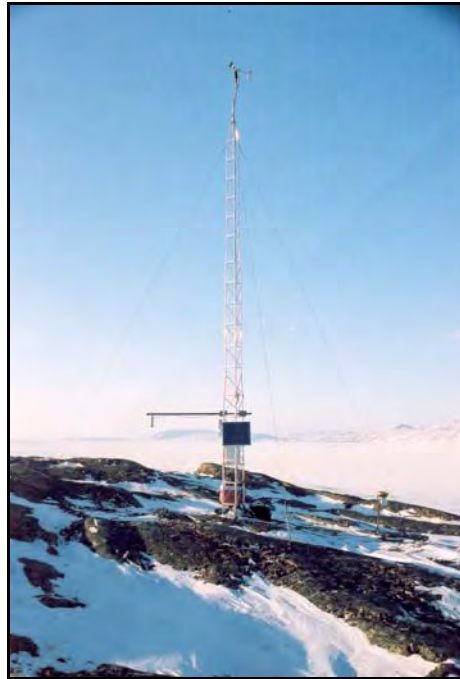
Plate 2.1-1. The Bathurst Inlet meteorological station (April 25, 2002). The 30 Watt solar panel and the cross arm for the SR50 Sonic Ranger (monitors snow depth) are about one quarter of the way up the tower. The RM Young 05305 wind monitor can be seen at the top.
