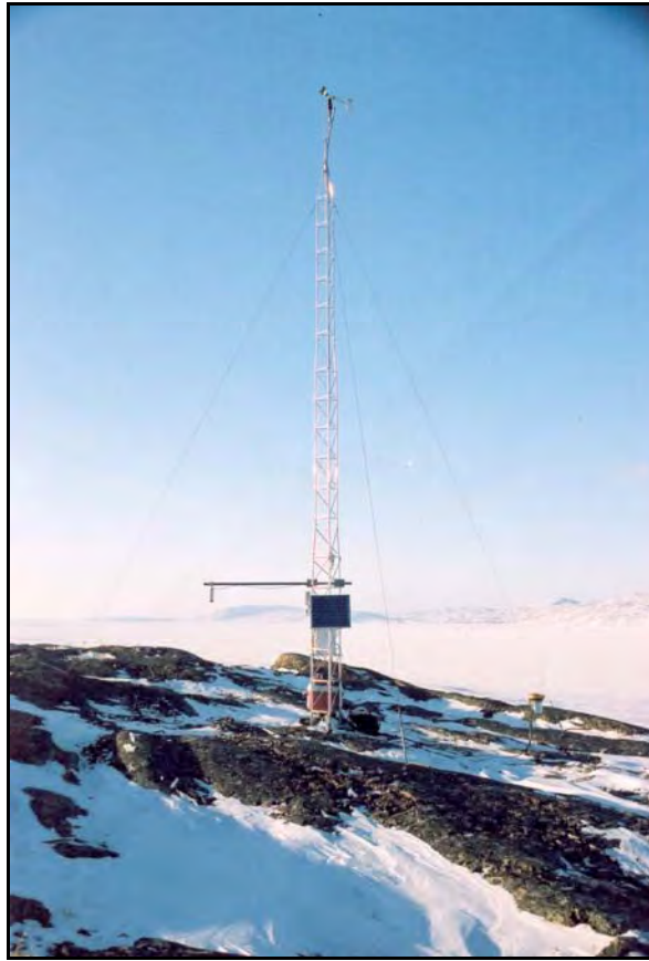
Plate 2.1-3 The Bathurst Inlet meteorological station was visited on April 25, 2002. The 30 Watt solar panel and the cross arm for the SR50 Sonic Ranger (monitors snow depth) are clearly visible about one quarter of the way up the tower. The RM Young 05305 wind monitor can be seen at the top of the tower
