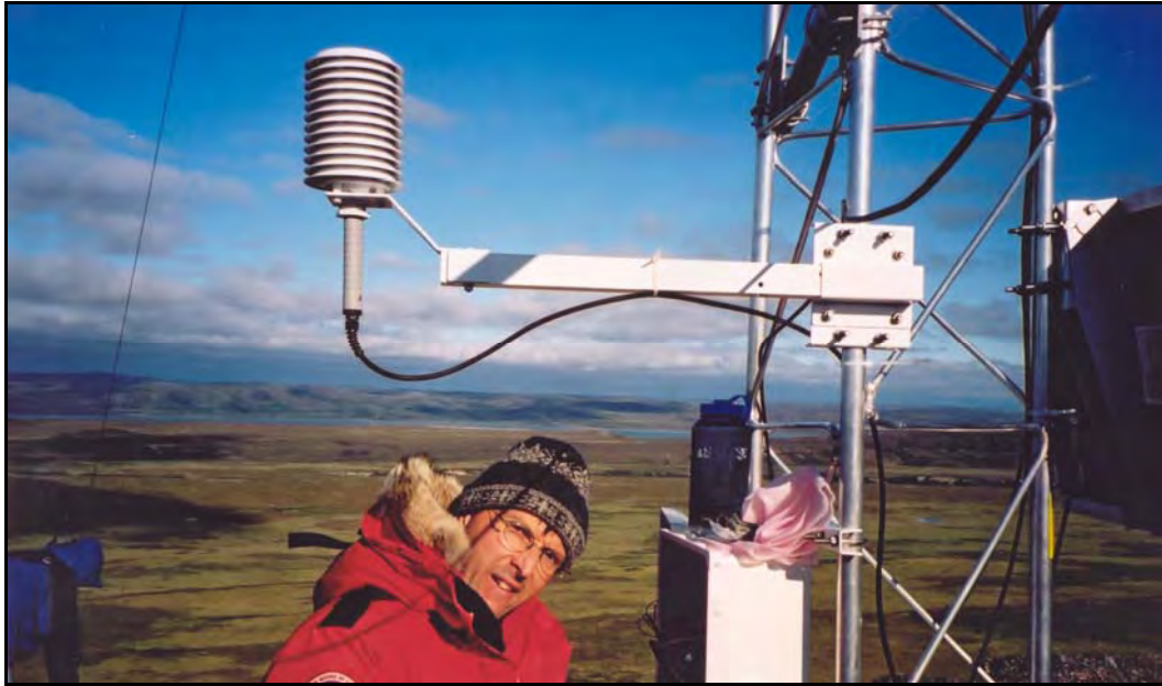
Plate 2.1-2 The white fiberglass box for the CR10X datalogger and the 12 plate Gill radiation shield for the temperature and relative humidity probe are shown in this photograph. Bathurst Inlet is visible in the background of the photo.
