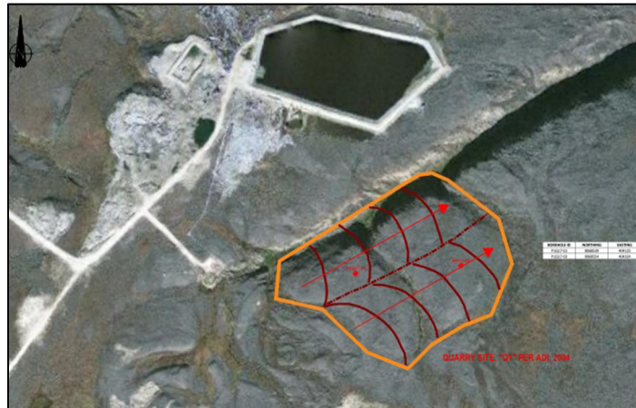
Sketch 5: Example of blasting sequence (Note that this sequence may change on field)
