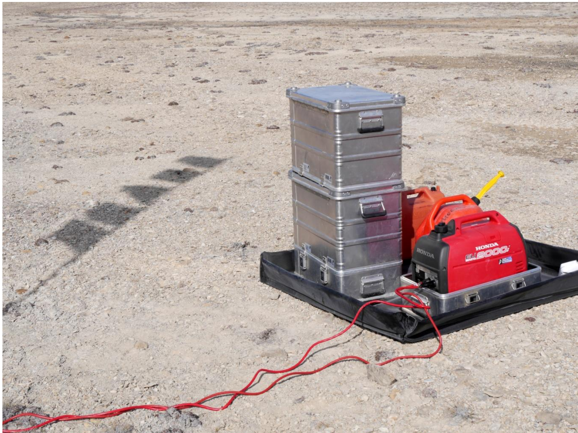
Generator with corresponding fuel in small berm behind the office tent. Spill kit not visible.
