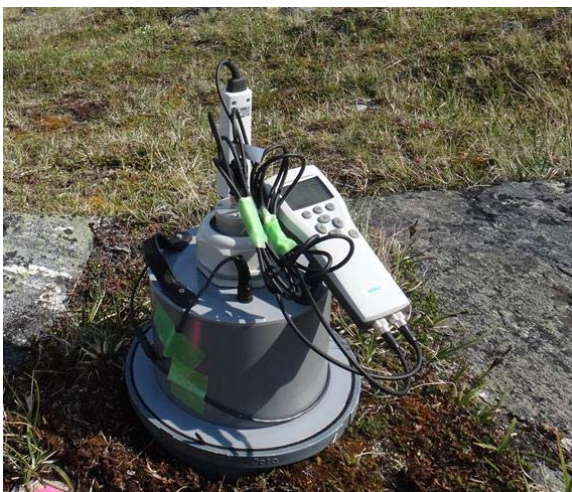
Photo 3. A non-destructive and non-disruptive carbon dioxide flux measurement.
