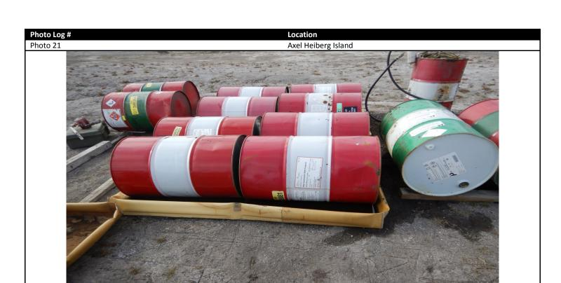
Description: 8 drums in secondary containment. Water from berm may of poured out during transfer of drums in and out of secondary containment
