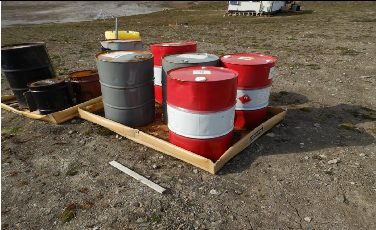
Description: Fuel Cache with secondary containment. And Spill kit
