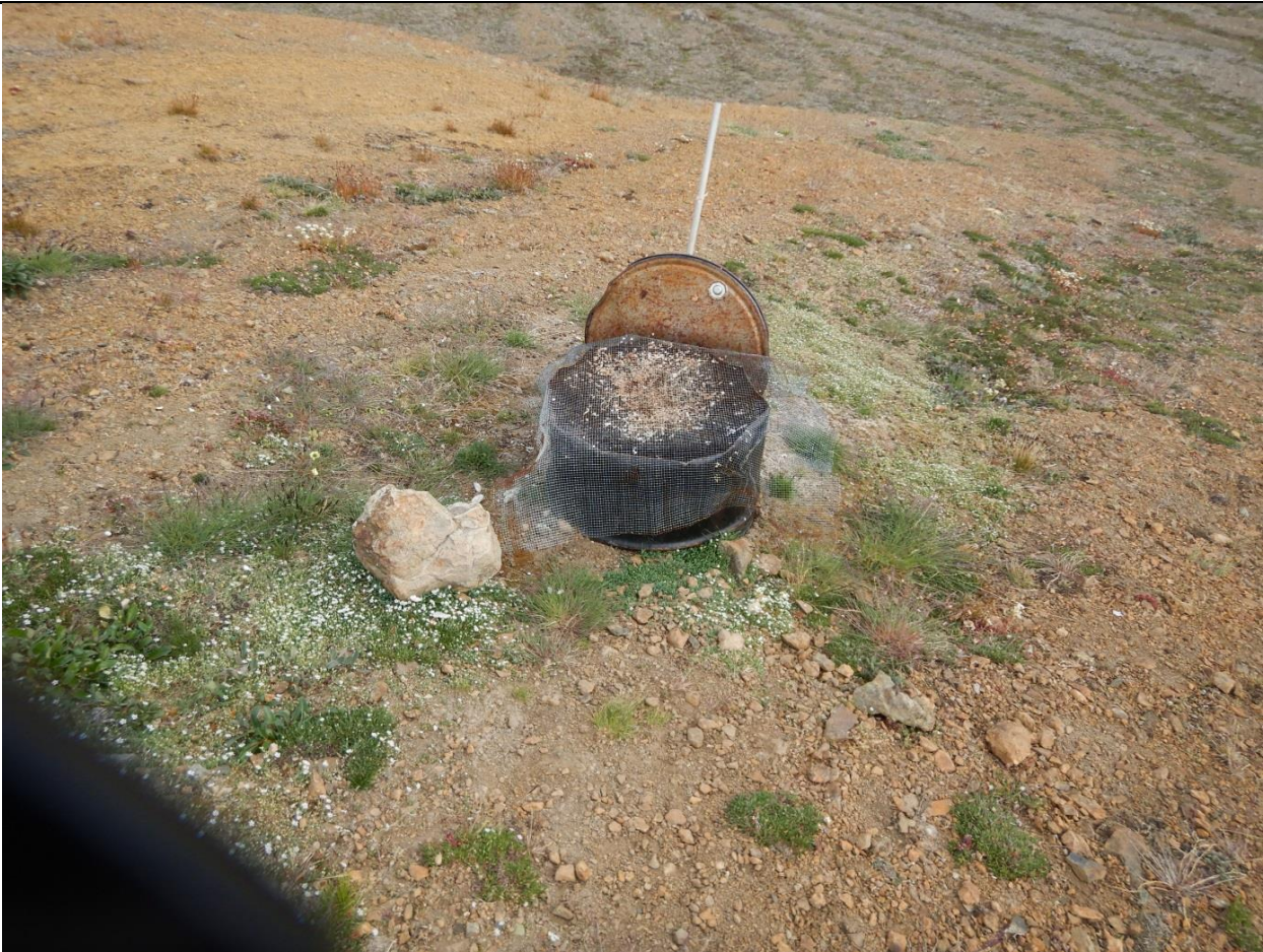
Description: Burn box – drum cut in half, mesh screen overtop to mitigate
