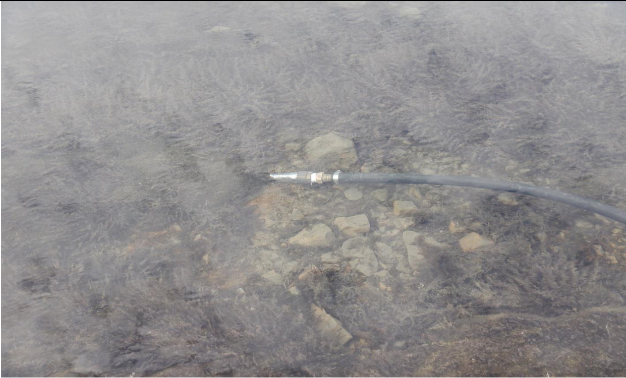
Description: Water Withdrawal hose, with fish mesh screen
