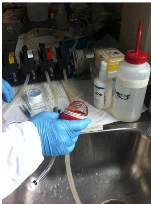
Fig. 3. Filtration and other manipulation of sample water in the laboratory before freezing the samples for subsequent analyses at UQAC and at Université Laval.
