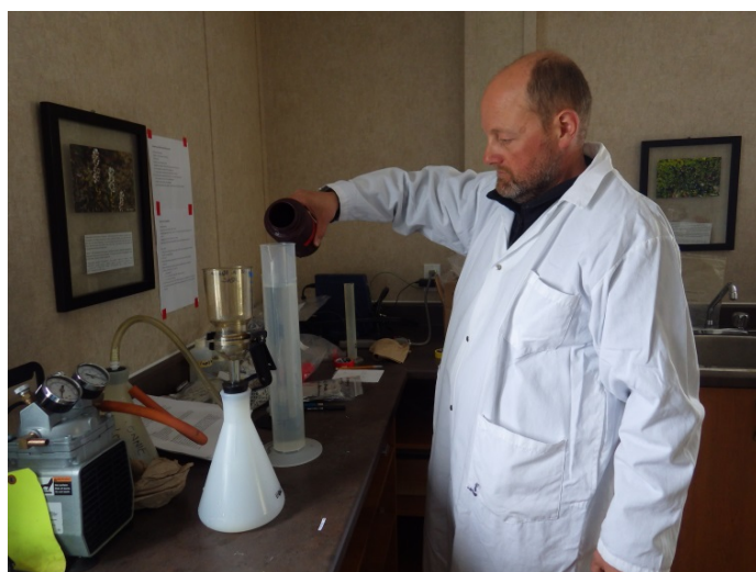
Fig. 3. Filtration and other manipulation of sample water in the laboratory before freezing the samples for subsequent analyses at UQAC and at Université Laval.
