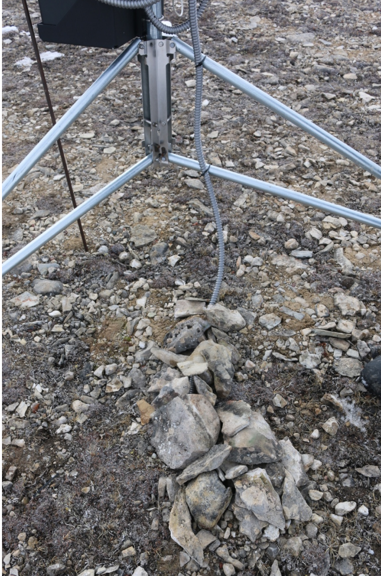
Figure 3. Soil temperature sensor cable, protected by metallic armour and rocks from arctic fox damage
