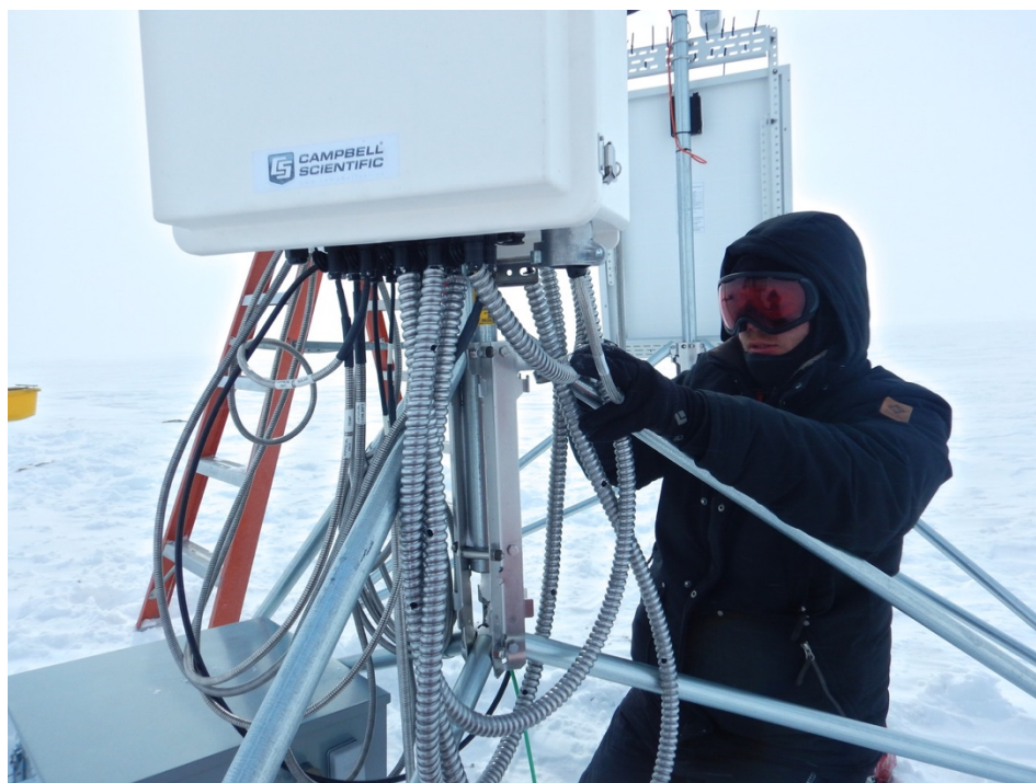
Figure 4. Armoured cables on the POLAR weather station in May 2018
