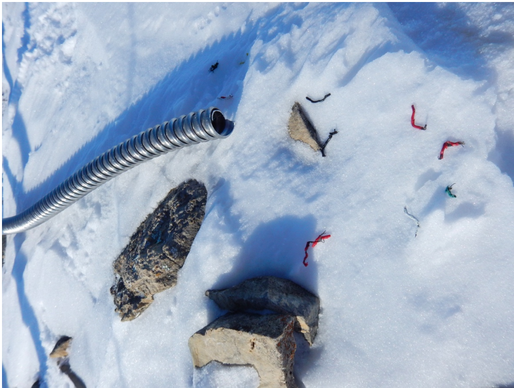
Figure 3. Cable damage caused by arctic foxes on the Université de Sherbrook weather station in April 2018
