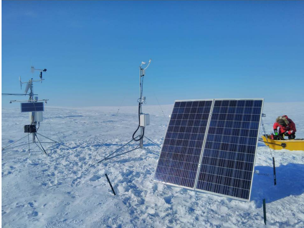
Figure 2. Disdrometer (background centre) and its solar panel array (foreground) installed in April 2018 as part of the Université de Sherbrooke weather station (background left).
