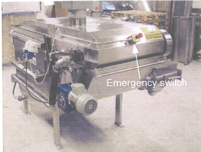
Picture 4: Location emergency stop button
